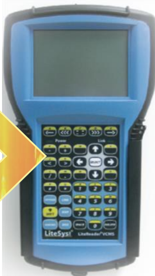
The Keypad Controller is designed to create, edit, and display messages.
